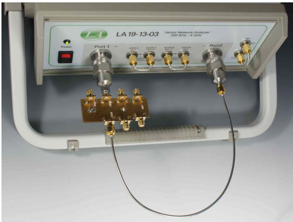
Figure 7. Measuring the test jig with the LA19-13-03
