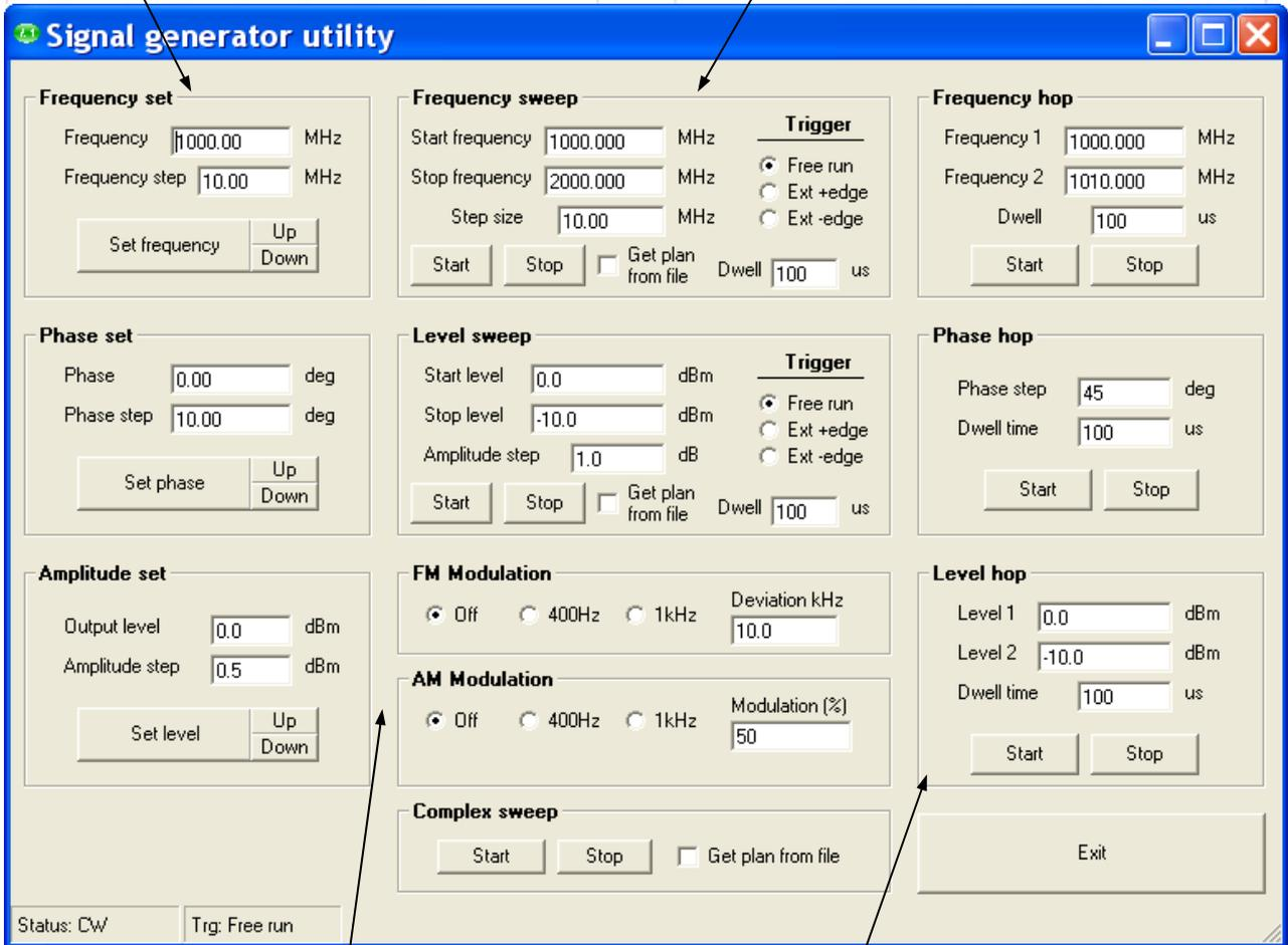
**FM and AM** modulation modes at 1 kHz or 400 Hz with up to 200 kHz FM deviation and up to 90% AM modulation depth.
